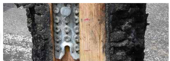
RICON® S connector after 90 minutes fire test. The wood is charred all around. The connector withstood the applied vertical load in the fire test.
