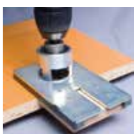
1a) Drilling with jig
