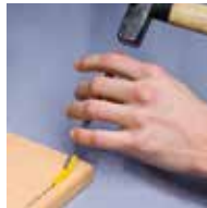
3) Knock in with the insert tool
