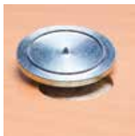
2) Mark counter part with center punch
