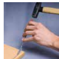
4) Knock in with the insert tool
