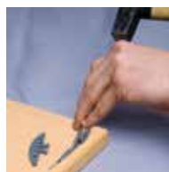
3) Knock-in with insertion tool
