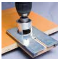
1a) Drill with jig
