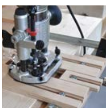
Mill with with routing-jig
