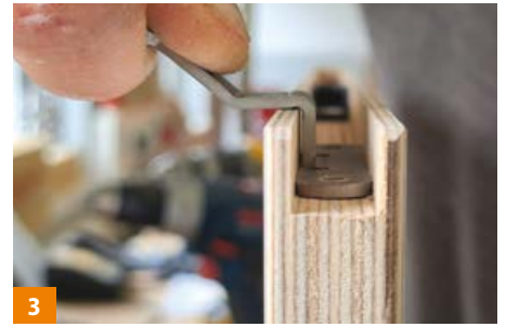
3 Position the drilling guide
