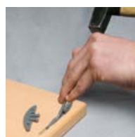
Knock-in with the insert tool
