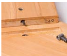
Insert clamping elements in holes
