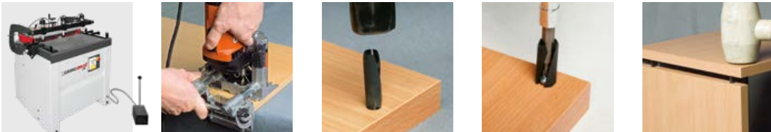
Drill with doweling machine or doweling joiner Knock in or screw Assemble
