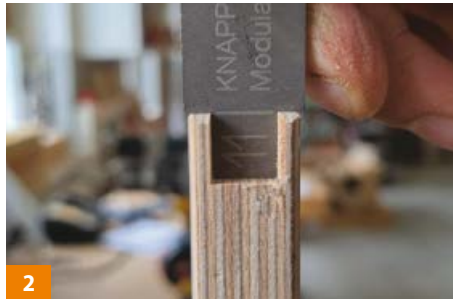
2 Check using the drill and test-jig
