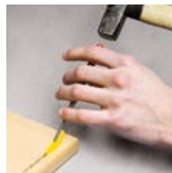
Knock-in with the insert tool
