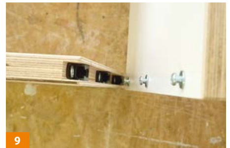
9 Attach the MODULAR pieces together.
