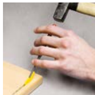
Knock-in with the insert tool
