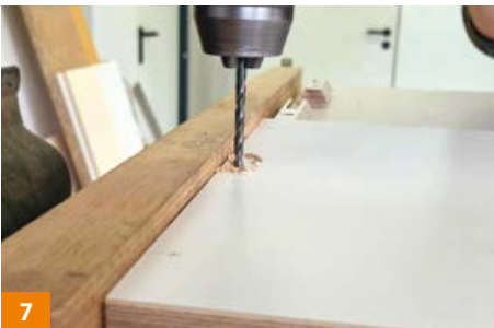
7 Drill holes for the shoulder-head screws.
