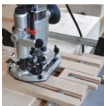
Mill with with routing-jig
