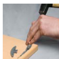
Knock-in with the insert tool
