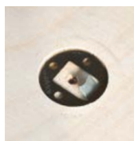
Install the locking clip to secure the assembly
