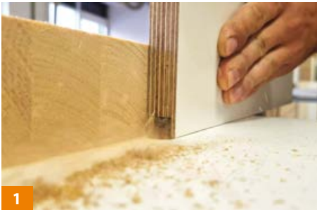
1 Mill the panels to the desired depth
