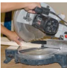
Cut to size glazing bead and FIXclip-profile
