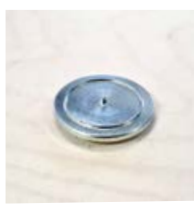
Mark counter part drilling position with centre punch
