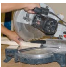
Cut to size glazing bead and FIXclip-profile
