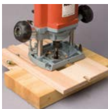
Route mortise with plunge router and routing jig.
