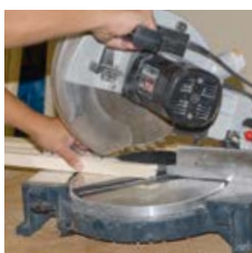
Cut to size glazing bead and FIXclip-profile
