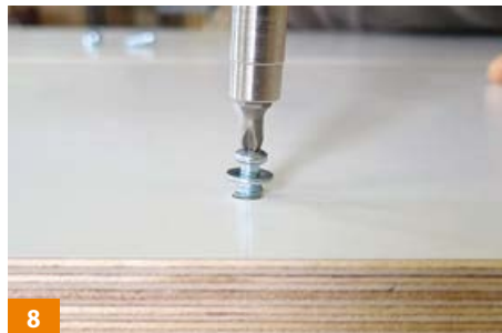
8 Screw in the shoulder-head screws.
