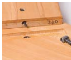
Insert clamping elements in holes
