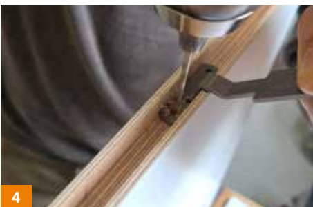
4 Drill holes using the drilling guides.
