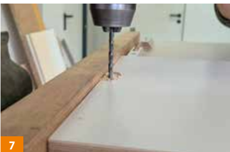
7 Drill holes for shoulder head screws.
