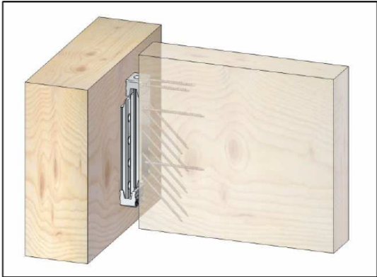
Header with joist 1: hang in joist
