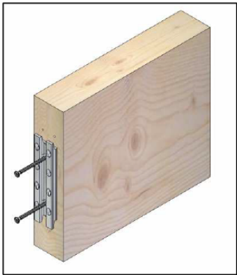
Joist 1: positioning screws
