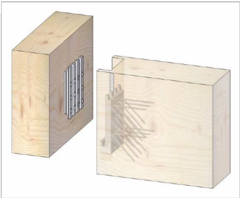
Header with joist 1: hang in joist
