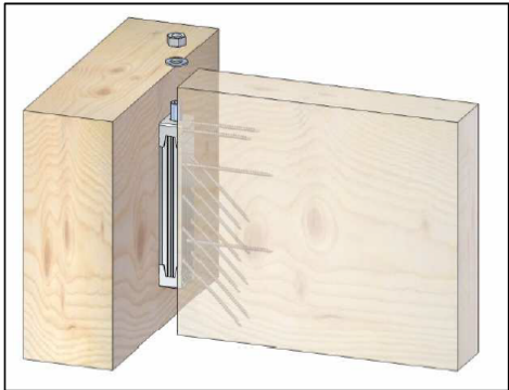
Header with joist 4: washer and hex nut
