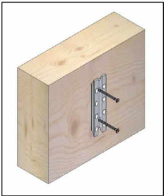
Header 1: positioning screws
