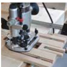
Mill with with routing-jig
