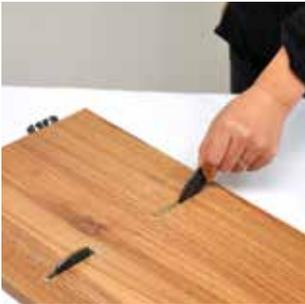
Insert the connectors flush with the panel.
