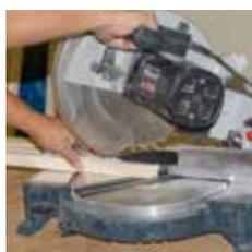
Cut to size glazing bead and FIXclip-profile
