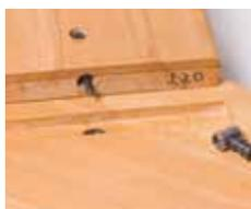
Insert clamping elements in holes
