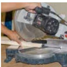
Cut to size glazing bead and FIXclip-profile
