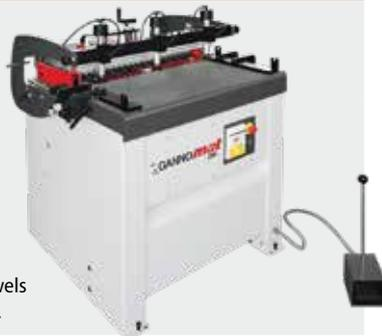
Dowel drilling based on KNAPP® dowels machining and conventional dowels.
