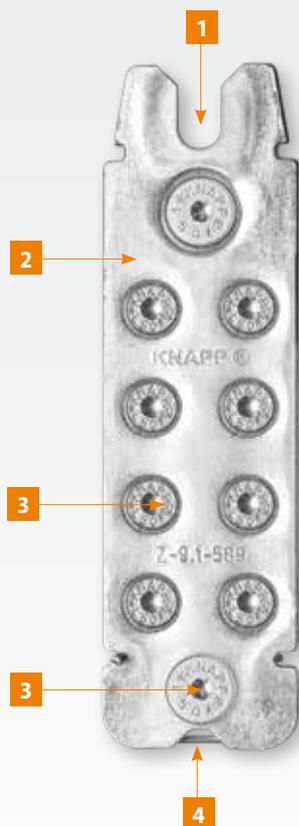
**1** The dovetail shape ensures optimum reception of the RICON® retaining CS-screws. The short clamping distance makes it easy to hook in, while engaging the plates, ensuring tightness and fast assembly of the elements.
