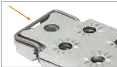
To unlock the connection, it is necessary to bend up the locking clip in its center e.g. with a screwdriver.
