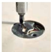
Position the connector using the holding tips
