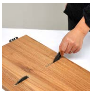
Insert the connectors flush with the panel.
