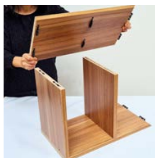
Assemble the components by fitting them together using hand pressure or a rubber hammer.
