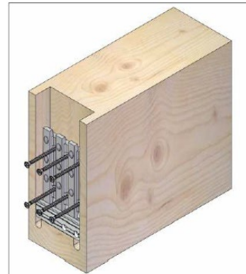
Joist 2: positioning screws
