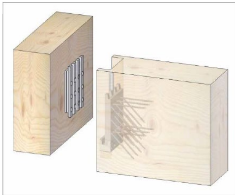
Header with joist 1: hang in joist
