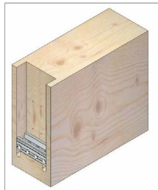
Joist 1: bottom clamping jaw in milling groove
