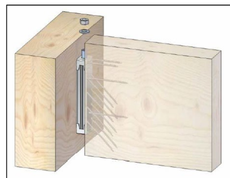
Header with joist 4: washer and hex nut
