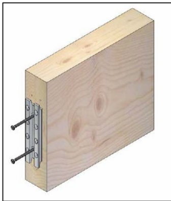
Joist 1: positioning screws
