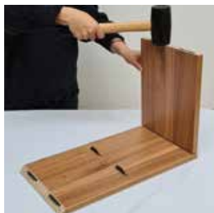
Use a rubber hammer to release the self-tightening mechanism.
