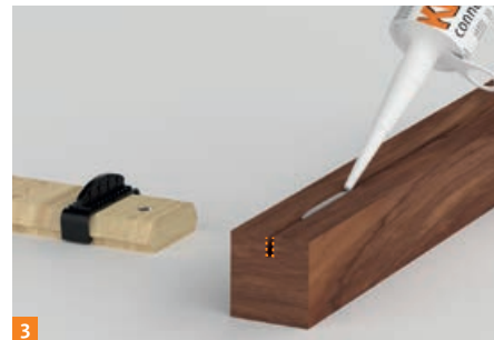
3 Mill a 4x12 mm groove and fill it with KNAPP® PU+ adhesive or apply the adhesive on the block rail. Fix the decorative moulding onto the block rail.
