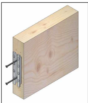
Joist 1: positioning screws
