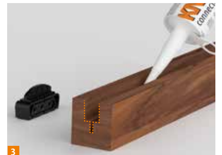
3 Mill a 2-level groove and fill it with KNAPP® PU+ adhesive or apply the adhesive on the block rail. Clip the workpiece onto the clamp.
