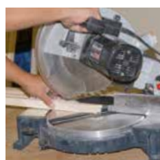
1) Cut to size glass bar and FIXclip-Profile
