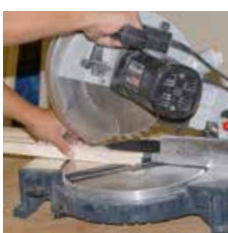
1) Cut to size glass bar and FIXclip-Profile
