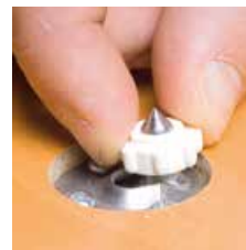
3) Transfer mark with center punch
