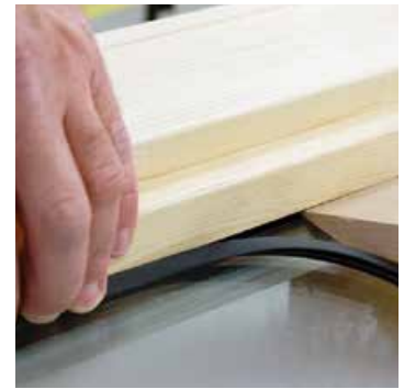
Press in wedge-shaped sealing
