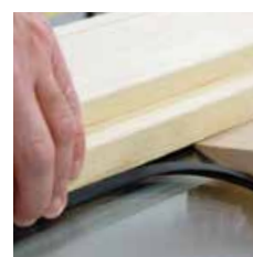
4) Press in wedge gasket sealing
