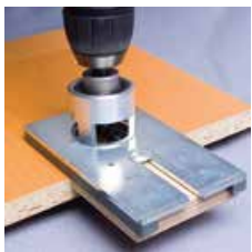
1A) Drilling with jig
