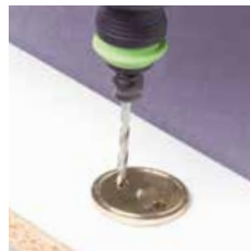
2) Transfer drill position with center punch. (make sure center is on the same line) and pre-drill with Ø = 5 mm, 12 mm deep.
