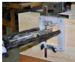
Drilling with stepped drill bit manual or with CNC.
