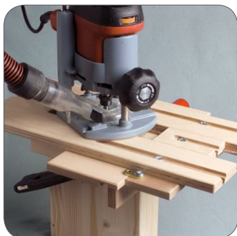
1) Routing with routing-jig and routing machine.
