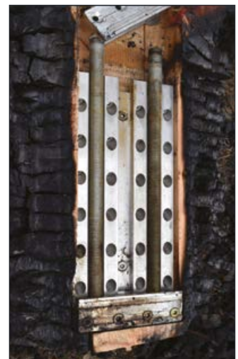
RICON®S connector after 120 minutes and MEGANT® connector after 60 minutes fire tests. The wood is charred all around. The connectors withstood the the vertical load applied in the fire test.
