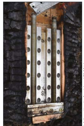
RICON®S connector after 120 minutes and MEGANT® connector after 60 minutes fire tests. The wood is charred all around. The connectors withstood the vertical load applied in the fire test.
