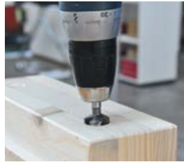
T-JOINT D20 Drill hole approx. 3 mm deep
