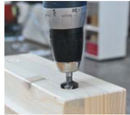
T-JOINT D20 Drill hole approx. 3 mm deep
