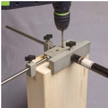
Pre-drill secondary beam
