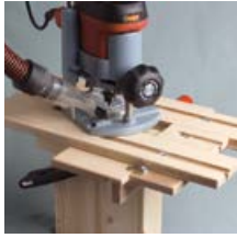
Recess with routing-jig
