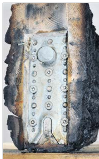
RICON®S connector after 120 minutes and MEGANT® connector after 60 minutes fire tests. The wood is charred all around. The connectors withstood the the vertical load applied in the fire test.
