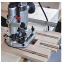
Mill with with routing-jig
